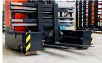
Different options for tyres make the truck extremely versatile: PU tyres are suitable for indoor use on industrial floors, PU SOFT tyres can be used both indoors and out, even on uneven floors and asphalt.
