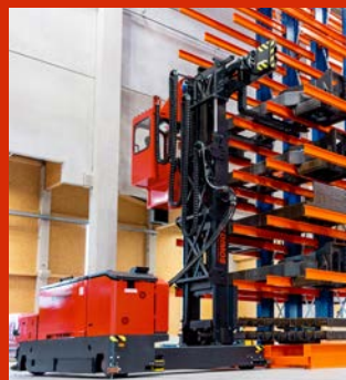
DMS with man-up cabin and unique initial lift system
