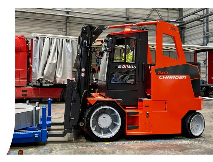
In the standard range, the drive is fully electric. Compared to an electro-hydrostatic drive concept, the efficiency of the truck is increased by 30%.
